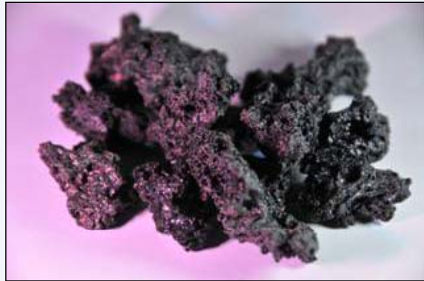
Basalt cinders from the Merriam Crater used to produce the JSC-1A family of simulants
